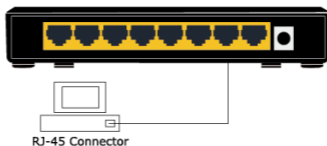
Switch connecting to an end node
